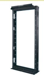
Ortronics Mighty Mo 110D Distribution Frame provides total vertical cable management to more effectively route cable in a 110 cross connect. Use with OR-30600166 to mount 100 or 300-pair blocks. Front and rear mounting supports up to 9000 pairs. Includes cable management straps in 165.1 mm deep vertical channels. Black.
