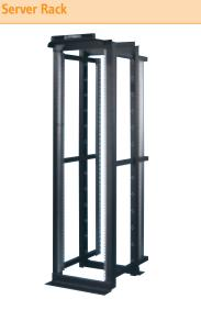
The mounting rails adjust from 152.4 mm to 812.8 mm, independent of the structural members. This makes it possible to mount "half height" rails on the frame, enabling equipment with different depth requirements to be mounted on one rack. Colour is black. Construction : Aluminium Frame with Steel EIA Rails, UL Listed.
