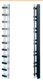
① Hinged latches allow easy access during moves, adds, and changes. 152.4 mm wide cage creates a 63.5 mm gap between racks for front-toback routing of equipment cables and patch cords.
